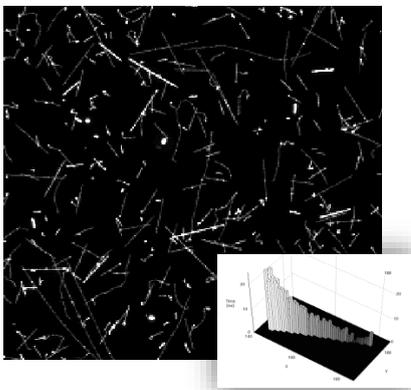
Illustration of single particle sensitivity of Timepix device. The tracks of different particles of radiation background (mostly muons and few protons) were recorded in 5 minutes on board of airplane. No noise (clean zero) is seen in dark regions. Inset shows the time profile along one muon track.
